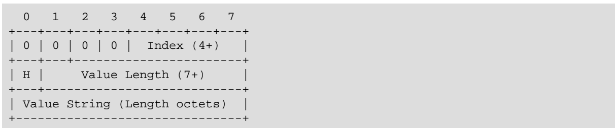
Figure 8: Literal Header Field without Indexing — Indexed Name
