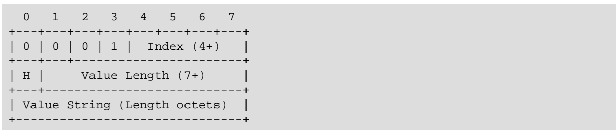
Figure 10: Literal Header Field Never Indexed — Indexed Name
