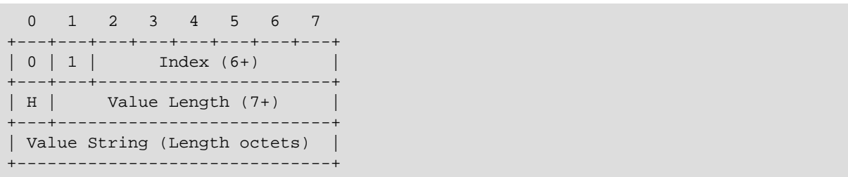
Figure 6: Literal Header Field with Incremental Indexing — Indexed Name
