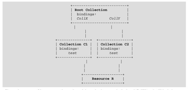
Given a host name of "www.example.com", applying a depth-zero write lock to "/CollX/test" will lock the resource R, and the lock-root of this lock will be "http://www.example.com/CollX/test".
